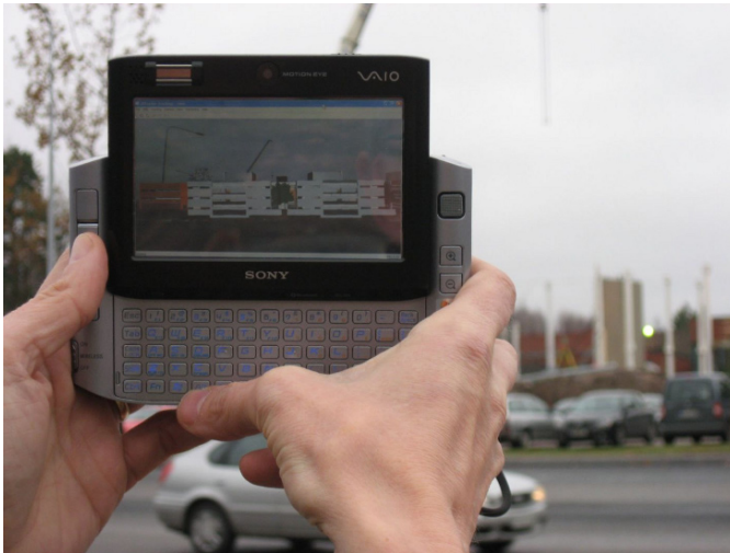
Fig. 15.4. Virtual building added to Google Earth, and visualized on site with a mobile device using AROnsite [214].
